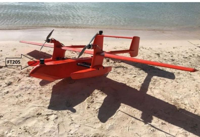
“The FT205 solved our problem just as we had hoped it would. Even when the drone landed on seawater, the data was not affected. The seawater appears to have had no effect on the sensor. Also, the accuracy of the data seemed to be higher than that gathered from a pitot tube, especially at low airspeeds – under 5m/s.
