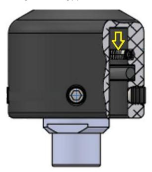
To facilitate a good connection please ensure any surface contamination or oxidation is removed from the mounting pipe prior to installation (this is easily achieved using Scotch Brite pads).
